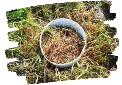
Infiltration set up: PVC ring located outside the Tiny Forest, ready for measuring
